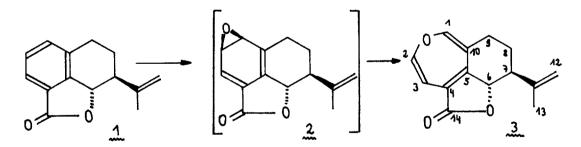
Most likely due to the presence of an electron acceptor and the two annellated saturated rings, $^{4,5,6}$ ) the equilibrium lies on the side of the oxepin, no trace of the arene oxide 2 was observed.<sup>2)</sup>
